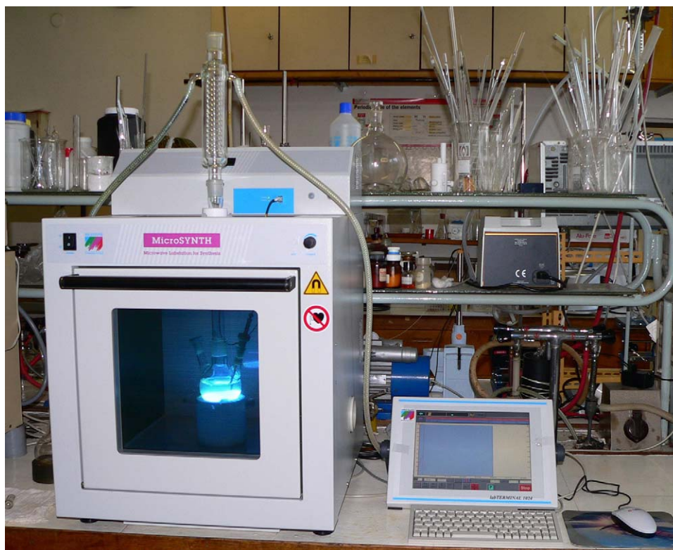
Fig. 2. Testing of the EDLs performance on Milestone's MicroSYNTH Labstation.
